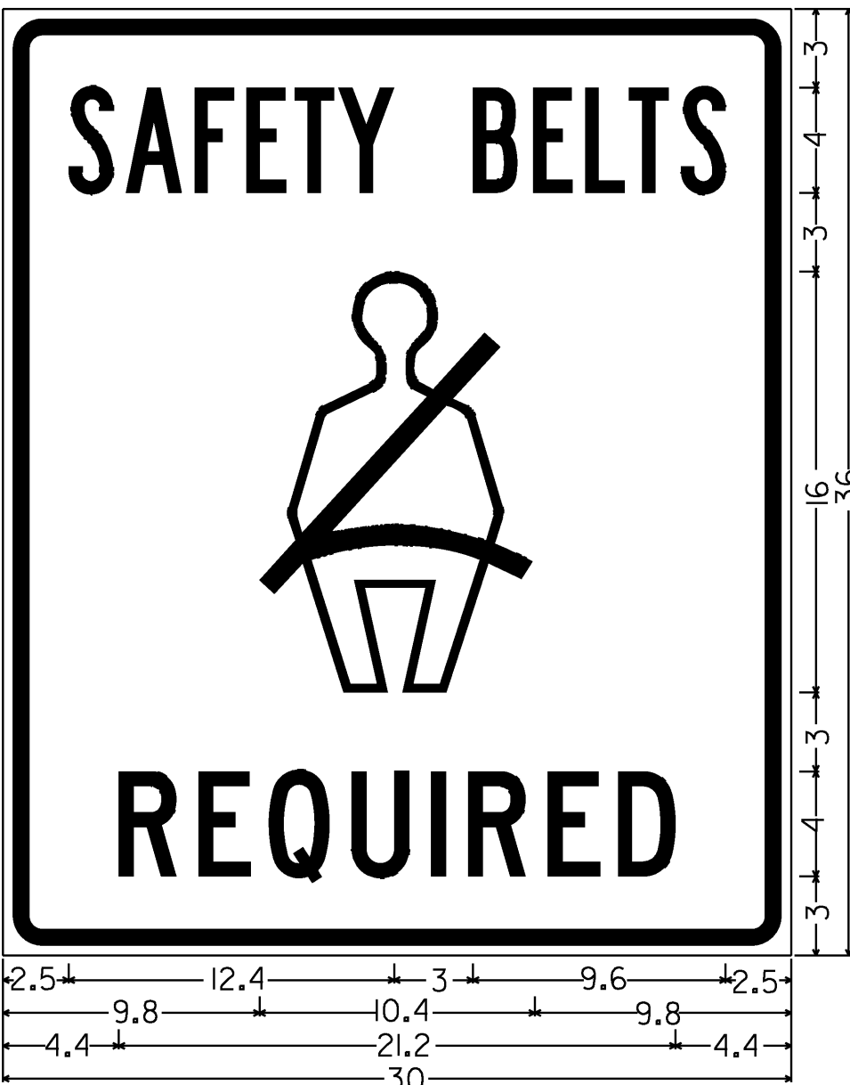
1.5" Radius, 0.6" Border, 0.4" Indent, Black on White; *SAFETY BELTS" B specified length; Symbol RG015; *REQUIRED" C;
