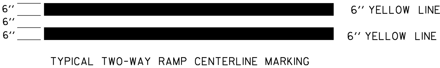
TYPICAL TWO-WAY RAMP CENTERLINE MARKING
