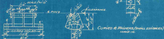
DETAIL LOWER HALF (SMALL EXR SHOE) MAKE 8 - STEEL CASTING. SCALE 1/2"=1'-0"
