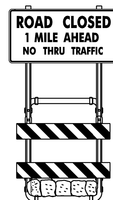
SIGN MOUNTING ON TYPE III BARRICADE (MODIFIED)
