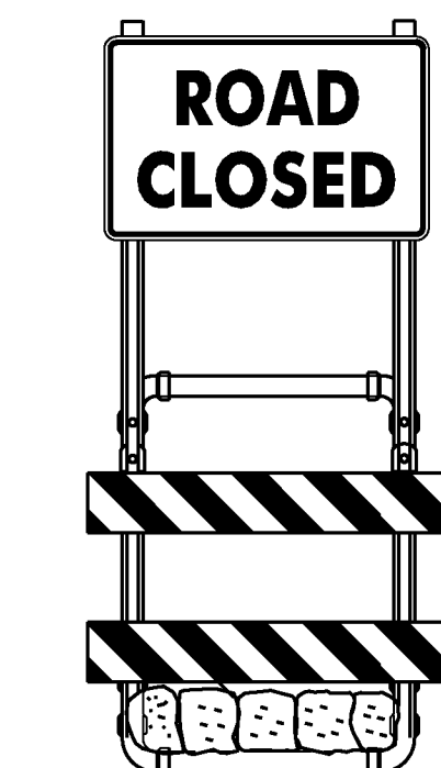
SIGN MOUNTING ON TYPE III BARRICADE (MODIFIED)
