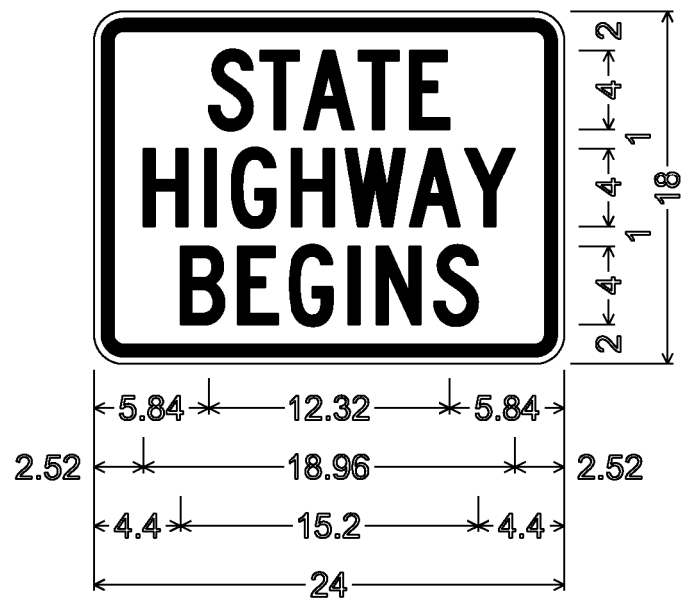
VR-039; 1.500" Radius, 0.625" Border, 0.375" Indent, Black on White; "STATE" C 2K; "HIGHWAY" C 2K; "BEGINS" C 2K;
