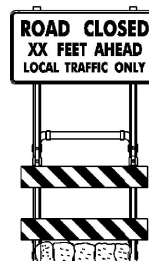
SIGN MOUNTING ON TYPE III BARRICADE (MODIFIED)
