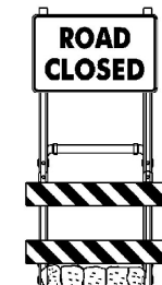
SIGN MOUNTING ON TYPE III BARRICADE (MODIFIED)
