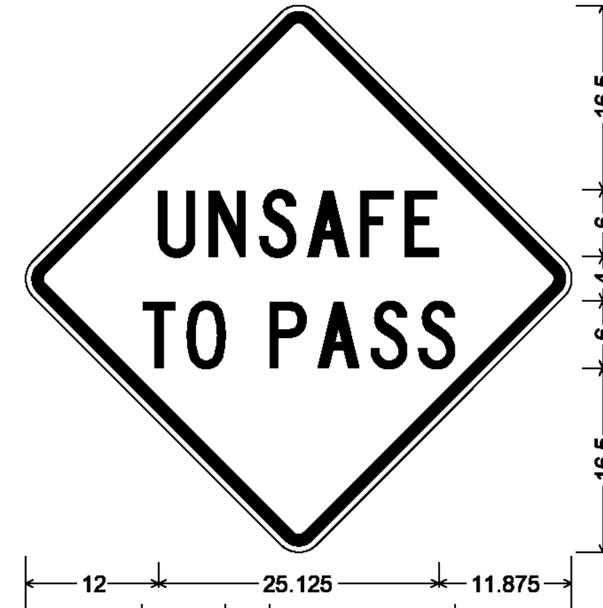
36.000" across sides 2.250" Radius, 0.875" Border, 0.625" Indent, Black on Yellow; [UNSAFE] C; [TO PASS] C; VW-092
