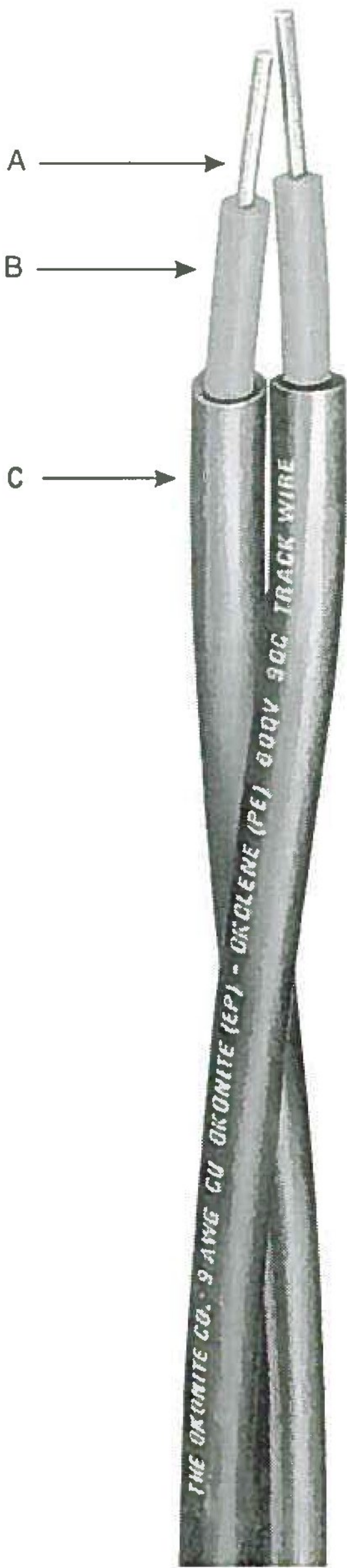
A Bare Copper Conductor- Size #9 AWG, #6 AWG Solid B Insulation - Okonite-Sizes #9 AWG and #8 AWG-5/64", #6 AWG-6/64" C Jacket-Okolene, Color Coded; 1-Black, 1-Red
