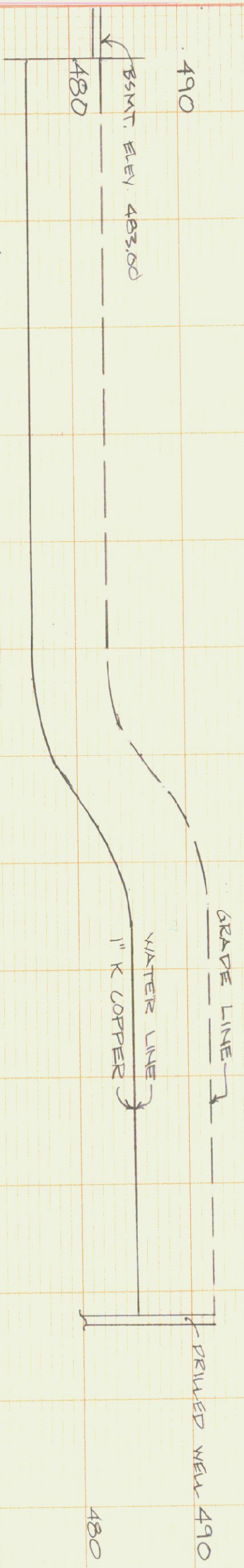
WATER LINE PROFILE OFFICE BLDG. TO WELL
